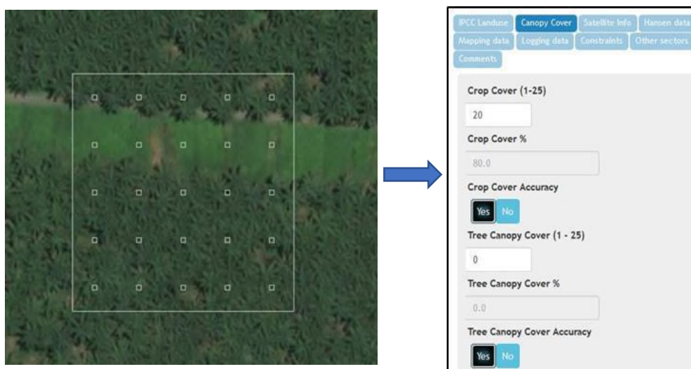
Figure 2-2. Example of measuring crop cover of a plot in a palm oil plantation
